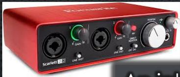
An interface (left) is necessary when using a conventional mic that has a standard XLR cable/connector
